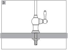
If necessary, tighten screws using a adjustable wrench until the faucet is firmly connected to the
